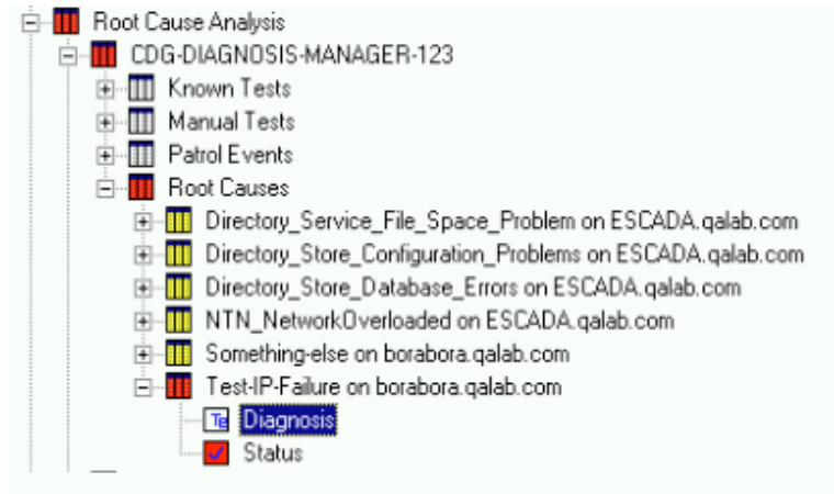
Figure 2 – This screen shot displays an exploded view of a diagnosis manager instance in the PATROL Console window.
