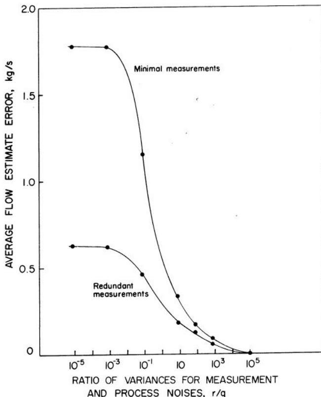
Fig. 4. Errors in flow estimates for blending network.
