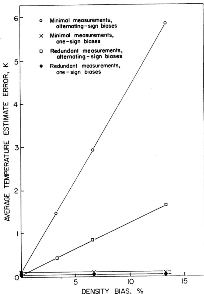
Fig. 8. Errors in temperature estimates for recycle network with density bias.
