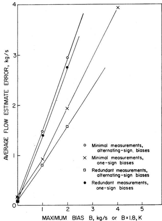
Fig. 7. Errors in flow estimates for recycle network with measurement bias.
